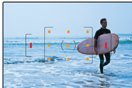
Nine cross-type sensors ( ) are positioned in the middle.
